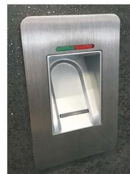
Biometric door lock with fingerprint sensor.
